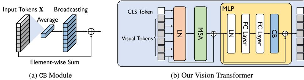
Figure 4: **Context Broadcasting (CB) module.** (a) Our CB module broadcasts the context to each token. (b) The CB module is inserted at the end of the MLP block of the Vision Transformer (ViT) architectures. ViTs have other possible positions for our module, but we analyze that inserting at the end of MLP outperforms others.
