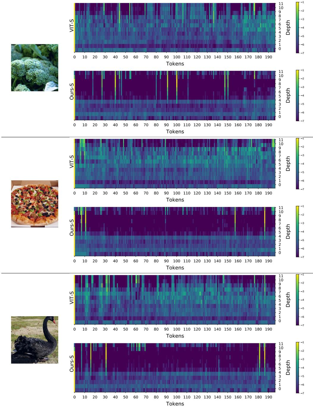
Figure 10: **Visualization of attention corresponding with the class token.**  $x$ -axis and  $y$ -axis represent tokens and depth. We denote ViT-S with CB as Ours-S. In ViT-S and Ours-S, the number of tokens and depth are 197 and 12, respectively; thus, the attention map is  $12 \times 197$ . We apply the element-wise log operation to attention for visualization.
